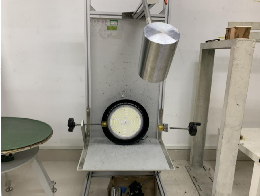
Photo 3: IK09 test of model GL-UFO200-C
